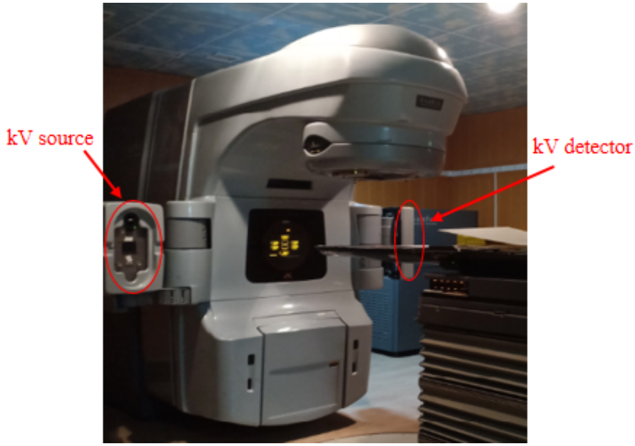
Figure 1.8: Illustration of a linac-mounted kV-CBCT system.
