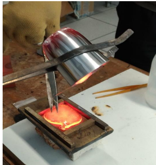
b) Poured onto pre-heated copper molds
