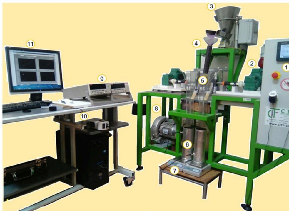
Fig. 1. Two-rotating disk-type tribo-aero-electrostatic separator. 1: Control panel. 2: Variable-speed dc motors. 3: Vibratory feeder. 4: Cylindrical feeder. 5: Separation chamber with two rotating disk electrodes. 6: Faraday cages. 7: Scales. 8: Air blower. 9: Electrometers (Keithley 6514). 10: Portable colorimeter NH310. 11: Computer [33].
