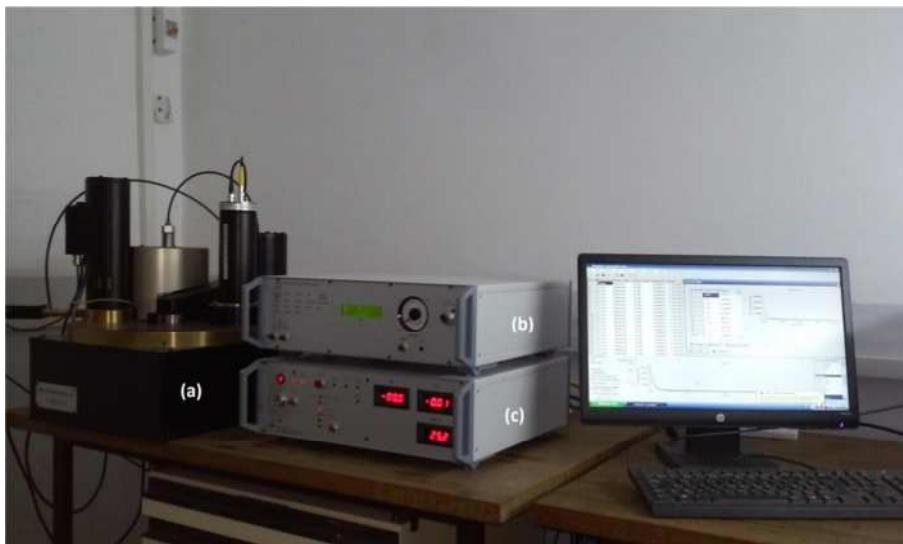
Fig. IV.3: RISØ TL/OSL-DA20 Reader, a) The Reader, b) The Controller, c) The X-ray generator controller
