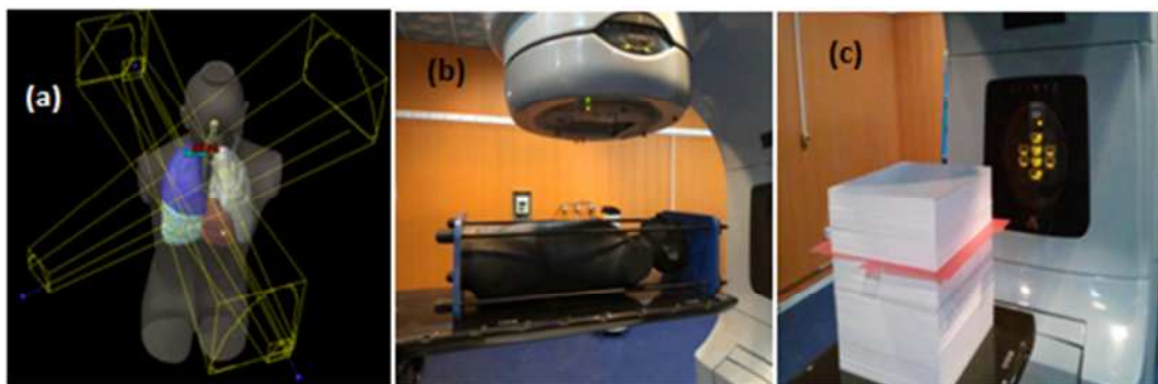
Fig IV.6: a) 3D Rando phantom image with the main treatment fields and lesion localisation (blue), b) Rando phantom placed on the radiotherapy Varian ClinacIX accelerator, c) water-equivalent RW3 slab phantoms used for TLD calibration
