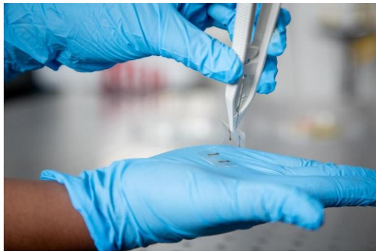
A sample of the ultra-thin and ultra-flexible electronic material that could be printed and rolled out like newspaper, for the touchscreens of the future. Source: RMIT University
