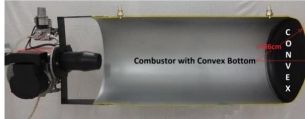
Fig. 4. Combustor with Convex Bottom (Case B)
