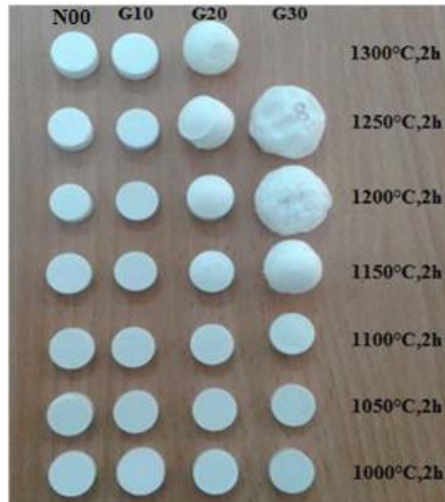
Figure 5. 1 samples sintered at different temperatures for 2 h
