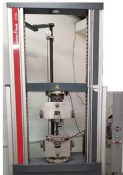
Figure III.15 Machine de traction Type : Zwick - 100
