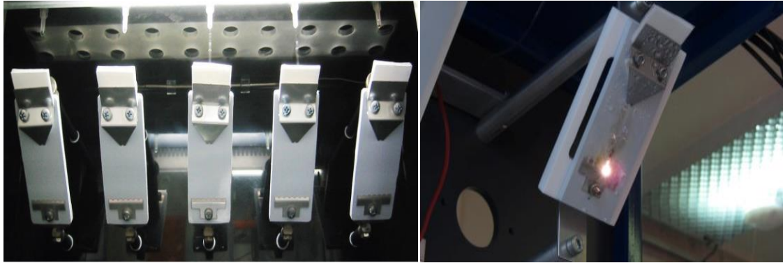
Figure 2.9 Test set-up for the inclined plane test according to the IEC 60587 standard [94].
