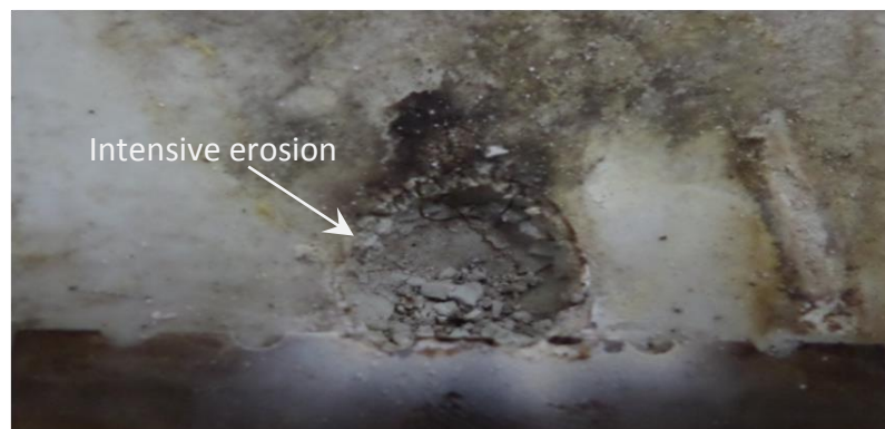
Figure 4.24 Close-up images of the eroded areas of non-textured sample tested at AC voltage
