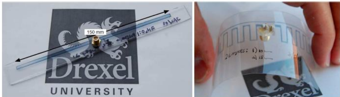
Figure 1.20. Two mechanically Flexible Antennas realized in PEDOT:PSS [30].
