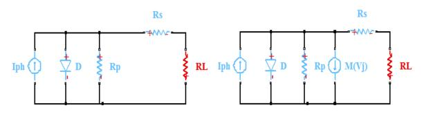
Figure 3.3: single diode model.Figure 3.4: Bishop model.
