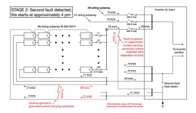
**Figure 2.5:** The second ground fault between an ungrounded current-carrying conductor (i.e., the positive conductor) and the equipment-grounding conductor.
