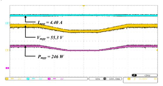
Figure 3.8: Voltage, Current, and Power curves measured by changing temperature, where *configuration-1* is used.
