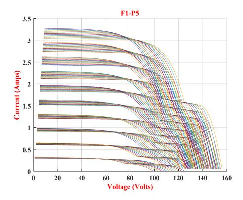
Figure 6: *I-V* curves for shading *pattern-5* (50% of nine PV cell in two PV modules).
