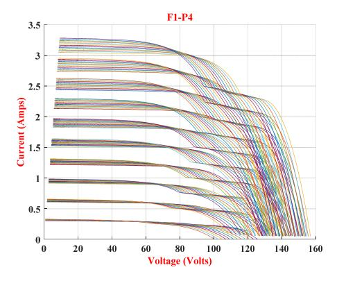
Figure 5: I-V curves for shading pattern-4 (25% of nine PV cell in two PV modules)
