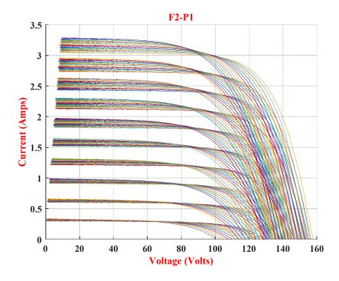
Figure 11: ISR *pattern-1* (the series resistance of one module is increased by 1  $\Omega$ ).
