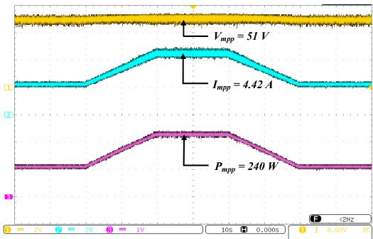
Figure 3.7: Voltage, Current, and Power curves measured by changing irradiance, where *configuration-1* is used.
