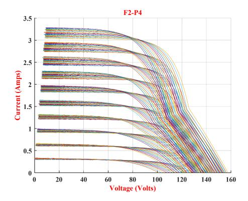
Figure 14: ISR *pattern-4* (the series resistance of one module is increased by  $15 \Omega$ ).
