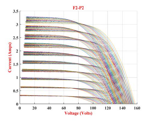
Figure 12: ISR *pattern-2* (the series resistance of one module is increased by 5  $\Omega$ ).
