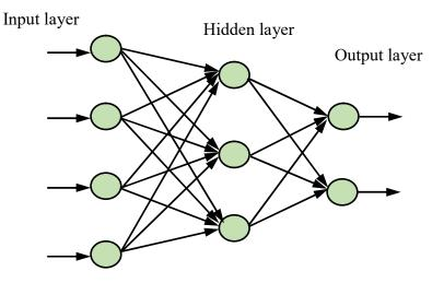
Figure .5.6: Multi-layer neural network concept.
