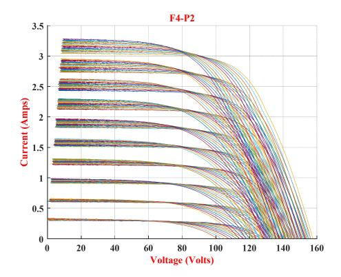
Figure 18: By-pass diode impedance (BPD is assimilated to a resistor of 5  $\Omega$ ).
