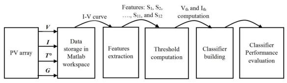
Figure .5.1: Process of classifier building for fault detection and classification in a PVA
