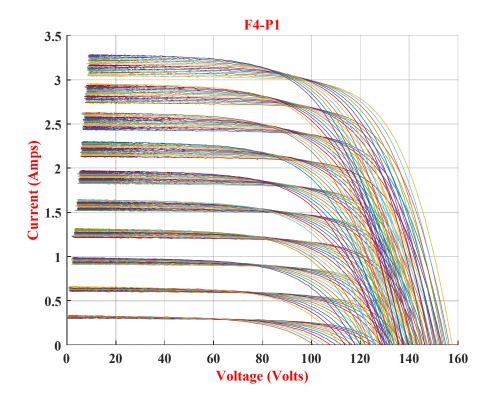
Figure 17: By-pass diode impedance (BPD is assimilated to a resistor of 1  $\Omega$ ).
