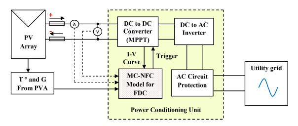
Figure .5.4: Schematic of the proposed FDC model for PVA.
