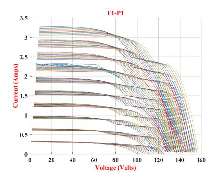
Figure 2: *I-V* curves for shading *pattern-1* (25% of nine PV cell in one PV module)
