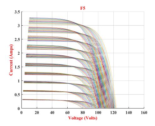
Figure 22: One PV module is short-circuited.
