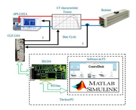
**Figure 3.1:** Schematic of the photovoltaic emulator with an APS61102A Programmable Power Source.
