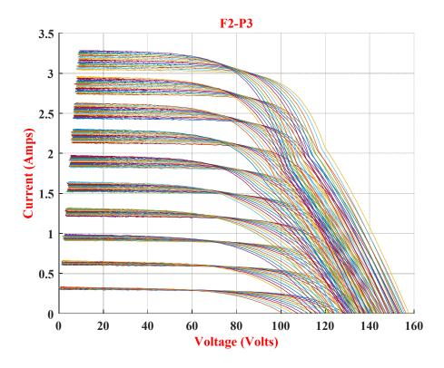
Figure 13: ISR *pattern-3* (the series resistance of one module is increased by  $10 \Omega$ ).
