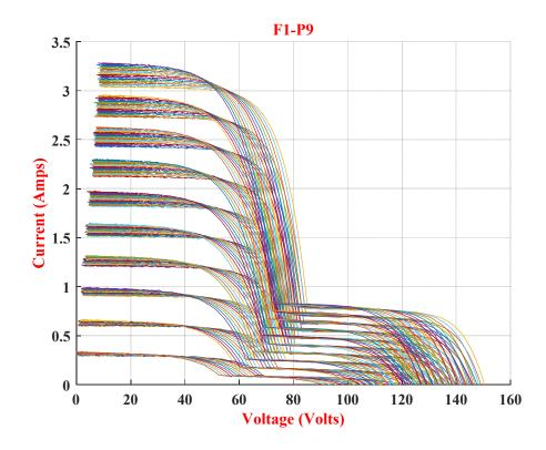
Figure 10: *I-V* curves for shading *pattern-9* (75% of nine PV cell in three PV modules)
