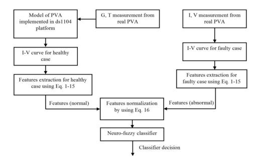
Figure 4.1: Overview of the proposed method for real-time fault detection and classification phase of unknown samples.
