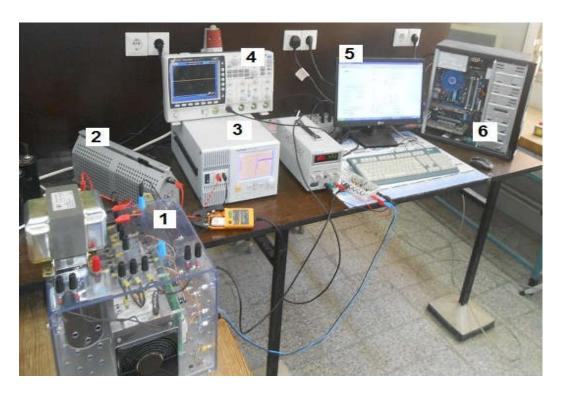
Figure 3.2: Photograph of the emulator used for data collection: 1) buck converters, 2) load,3) programmable power source, 4) scope, 5) ControlDesk, 6) ds1104 platform.
