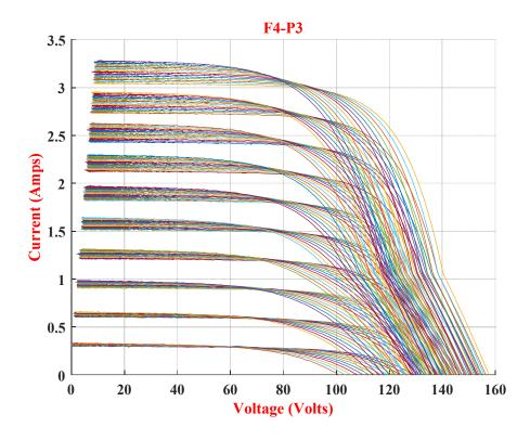
Figure 19: By-pass diode impedance (BPD is assimilated to a resistor of  $10 \Omega$ ).
