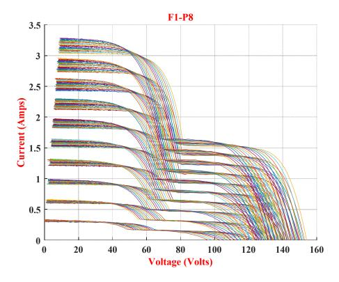
Figure 9.h: I-V curves for shading pattern-8 (50% of nine PV cell in three PV modules)
