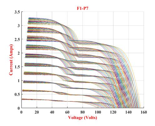
Figure 8: I-V curves for shading pattern-7 (25% of nine PV cell in three PV modules)
