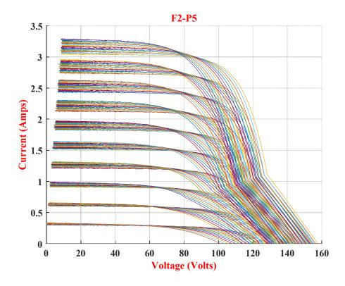
Figure 15: ISR *pattern-5* (the series resistance of one module is increased by  $20 \Omega$ ).
