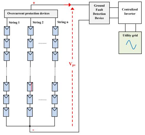
**Figure 6.1:** Schematic diagram of a typical grid-connected PV system, including conventional protection devices.
