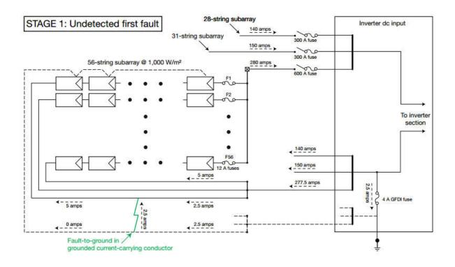
**Figure 2.4:** The first undetected ground fault between a grounded current-carrying conductor (i.e., the negative conductor) and the equipment-grounding conductor.
