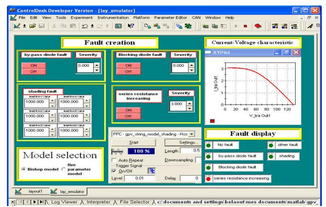
Figure 3.11: ControlDesk interface showing Increased Series Resistance condition, where *configuration-2* is used.
