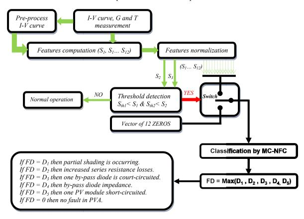
Figure 4.2: The structure of the fault detection and classification algorithm based on classifiers decision outputs fusion.
