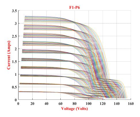
Figure 7: *I-V* curves for shading *pattern-6* (75% of nine PV cell in two PV modules).
