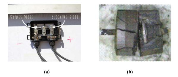
Figure 2.1: (a) good bypass diode and blocking diode, (b) damaged diode.
