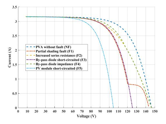
Figure 3.6: *I-V* curves of different PV array faults.
