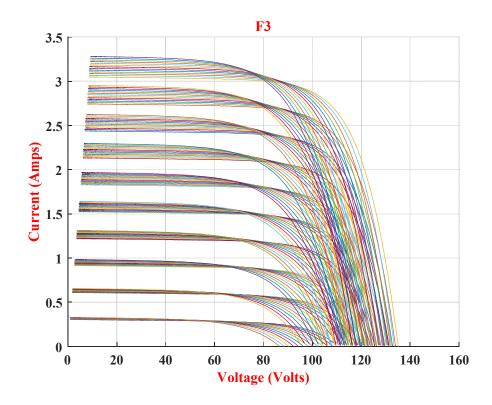
Figure 16: By-pass diode short-circuited (1 BPD in the whole PVA short-circuited).
