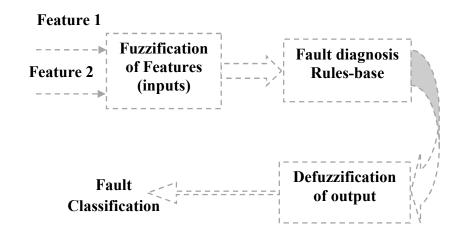
Figure .5.5: Fault Fuzzy classifier implementation concept.
