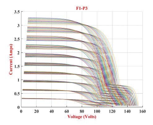
Figure 4: I-V curves for shading pattern-3 (75% of nine PV cell in one PV module)
