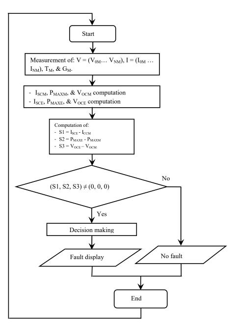
Figure 3.9: Flowchart of the diagnostic algorithm
