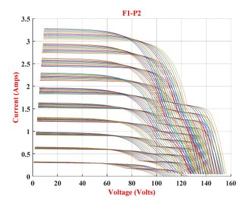
Figure 3: I-V curves for shading pattern-2 (50% of nine PV cell in one PV module)
