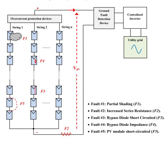
Figure 1.3: Schematic diagram of a grid-connected PV system, together with different types of faults in the PV array.
