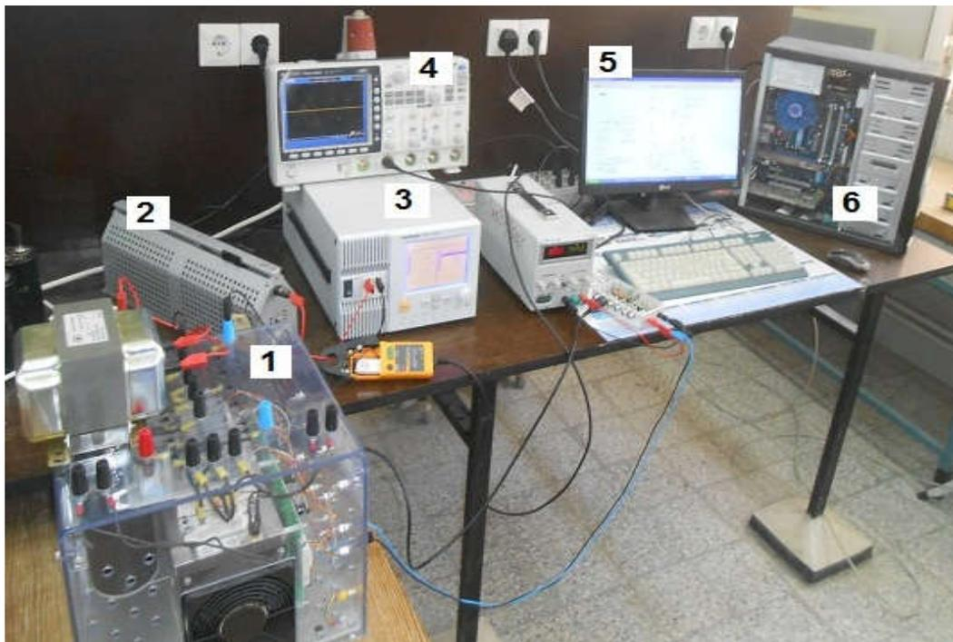
**Figure 3.2:** Photograph of the emulator used for data collection: 1) buck converters, 2) load, 3) programmable power source, 4) scope, 5) ControlDesk, 6) ds1104 platform.
