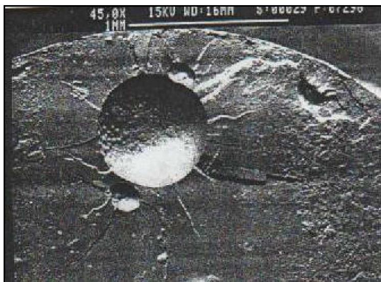
Figure II.14 SEM micrograph of fatigue fracture surface. The two small pores adjacent to the large pore caused stress concentrations which initiated several cracks.<sup>(96)</sup>
