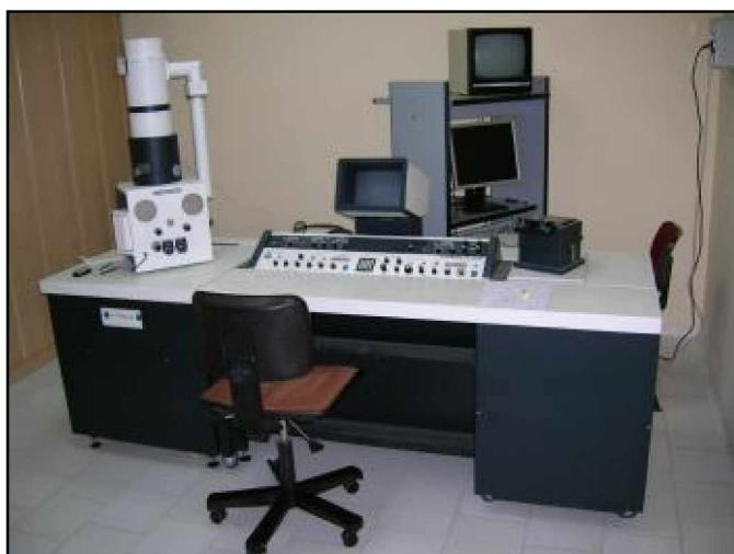
Figure III.17 SEM, StereoScan-200, Cambridge Instruments.
