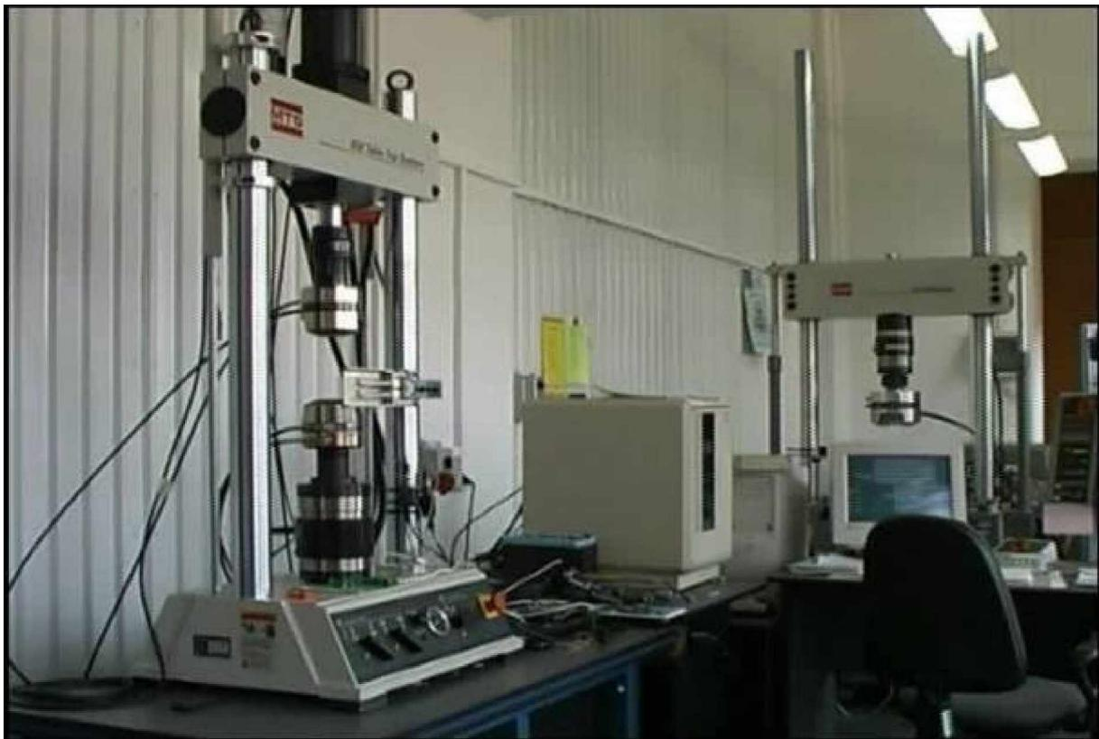
*Figure III.8* MiniBionix 858 testing machine.
