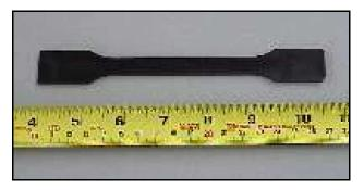
Figure II.1 A dog bone specimen used in tensile tests.
