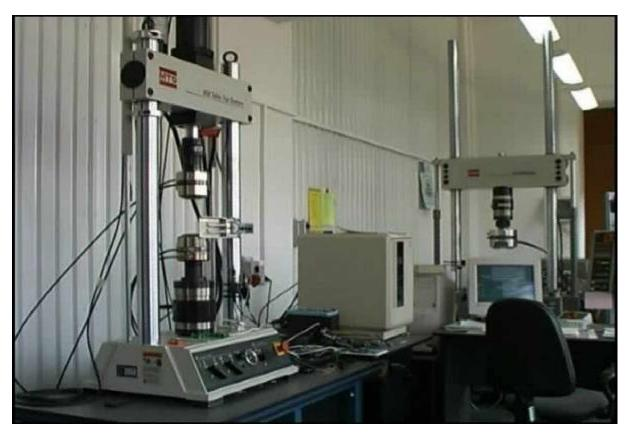
Figure III.8 MiniBionix 858 testing machine.
