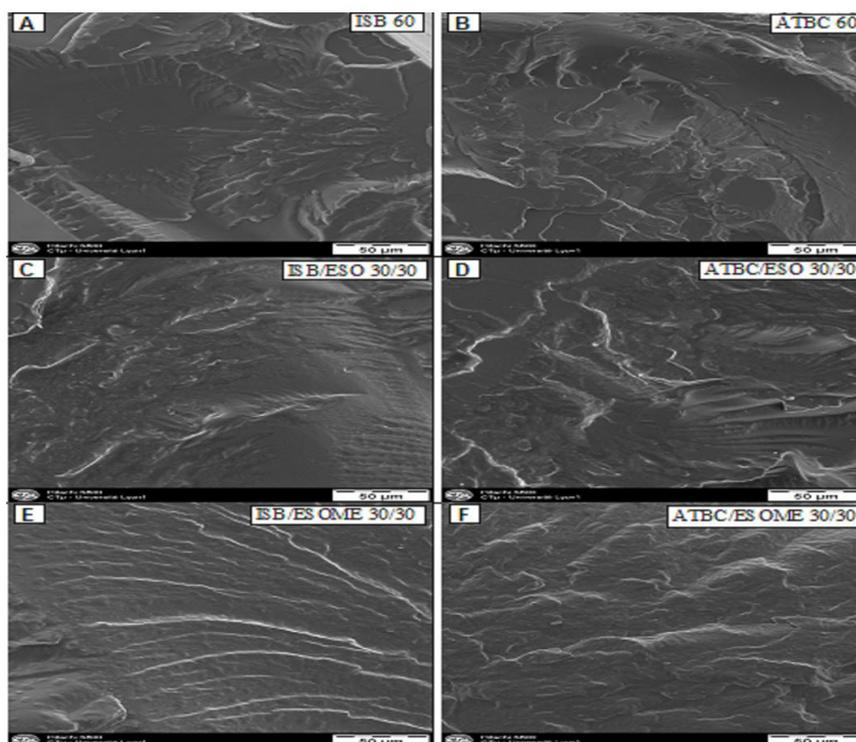
**Figure 7.** SEM micrographs of fracture surfaces of PVC films with different plasticizer compositions: (A) ISB 60 phr; (B) ATBC 60 phr; (C) ISB/ESO 30/30; (D) ATBC/ESO 30/30; (E) ISB/ESOME 30/30; (F) ATBC/ESOME 30/30.
