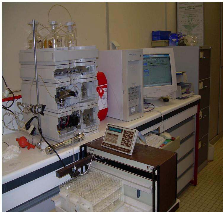
**Figure 10. Appareillage la CLHP**
