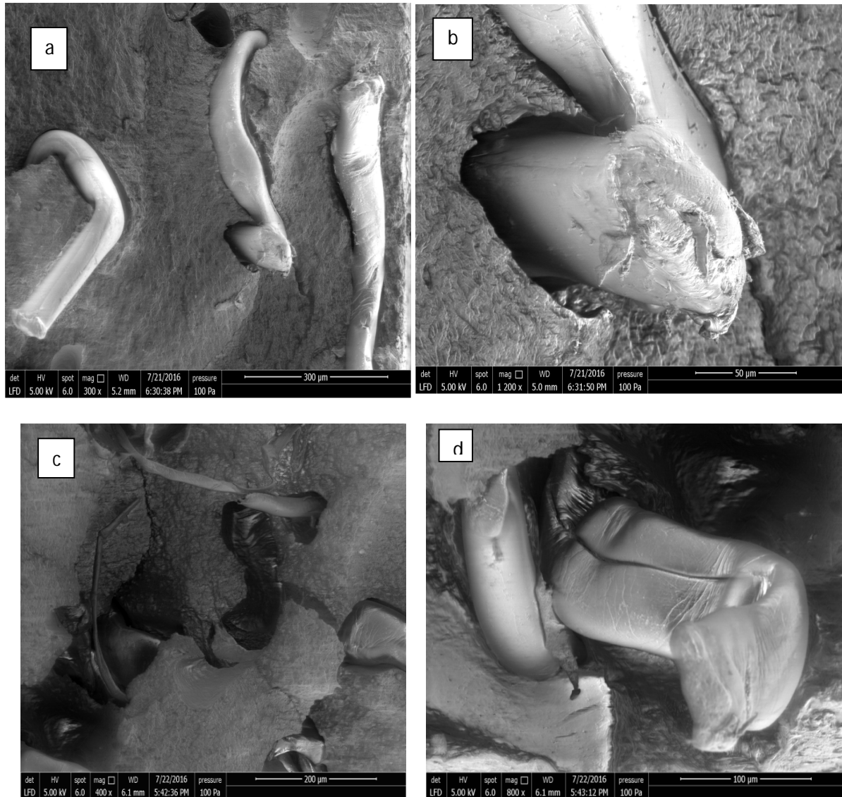
Figure IV.99. SEM micrographs of the tensile fractured surface of the untreated (a, b) and treated (c, d) 7 wt% PET fiber /PP composites
