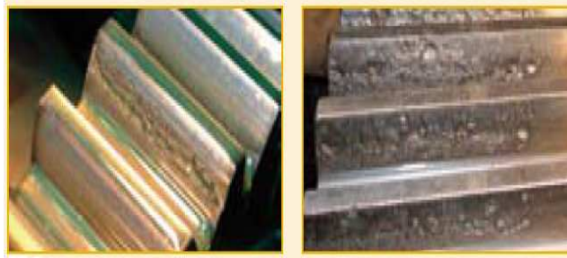
Figure I.18 Pitting ou piqures
