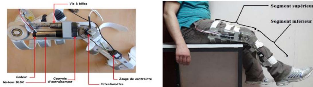
Figure 1.12: Exosquelette du LISSI
