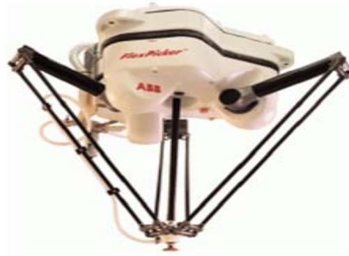
Figure 1.3: Robot Delta FlexPicker
