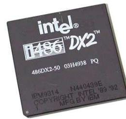
Figure 2.6 -  $\mu$ P Intel 486 DX2 50MHz
