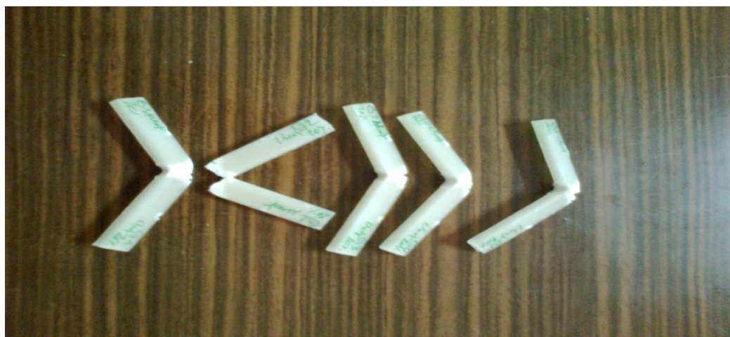
Figure VI.22 Representative Broken Samples of the PC-I Ternary Nanocomposites at 20 wt% Rubber Ratio.
