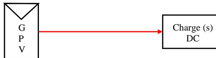
**Figure 1.21.** Couplage direct GPV-charge.
