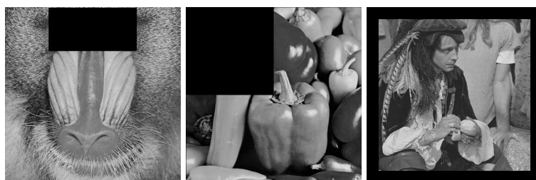
Figure 4.13: Robustness of the DWT-DCT technique against different type of cropping. The BCR values is 100\% for these attacks.
