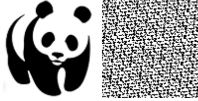
Figure 5.5: The binary watermark image and its scrambled version using Arnold transform.
