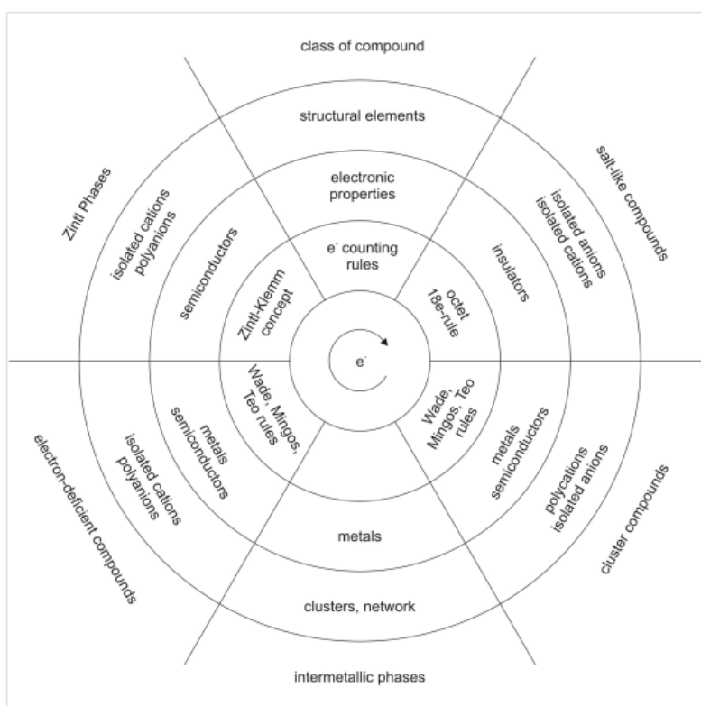
Fig I.2 Relations between classes of chemical compounds through the comparison of structural elements, electronic properties, and electron-counting rules [8].
