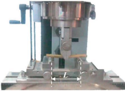
Fig. 1. Three point bending test set-up.
