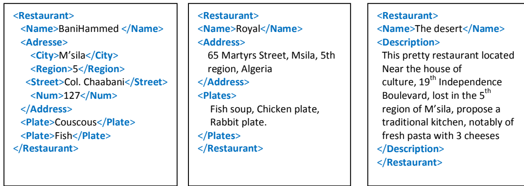
Figure 5.12. Three XML documents describing restaurants with different structures.
