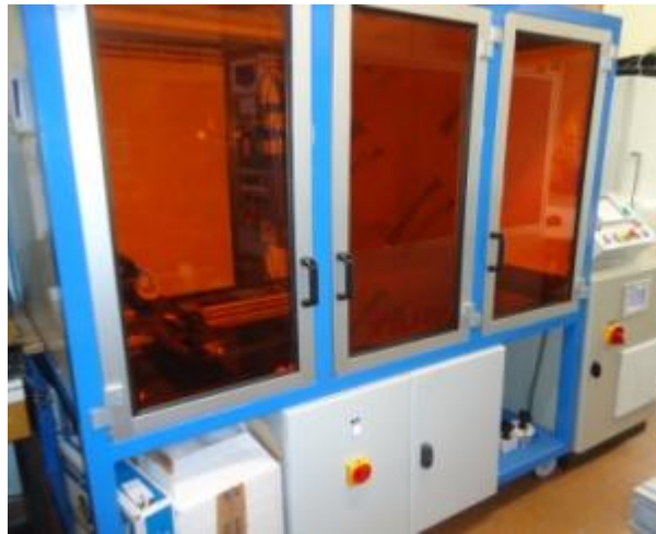
Figure 3-5: Photo of the Dr. Hönle UV lamp (UVH medium-pressure mercury arc lamp)
