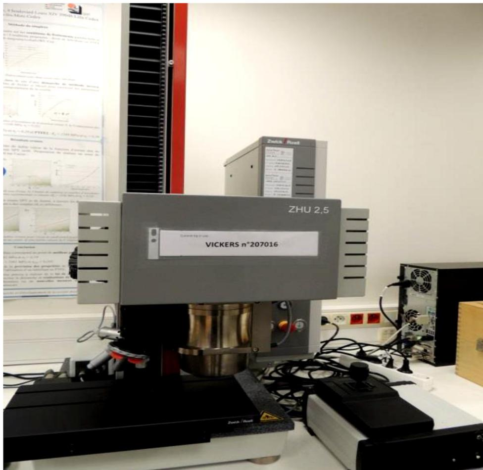
Figure 4.25: Machine d'indentation Zwick ZHU 2.5
