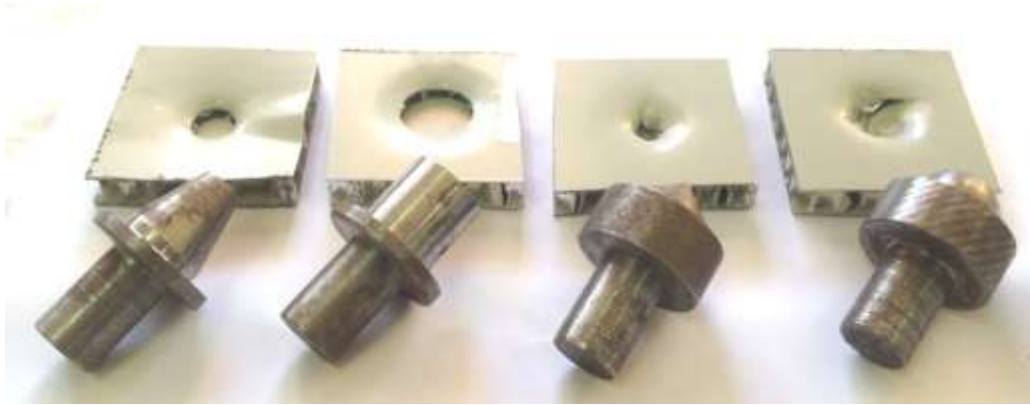
Figure 3.42: Failure modes of indentation test for each indenter.
