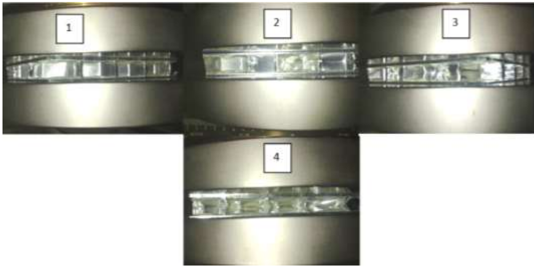
Figure 3.53: Stages of quasi-static compression test of aluminum honeycomb: (1) initial state, (2) buckling initiation, (3) progressive folding and (4) densification.
