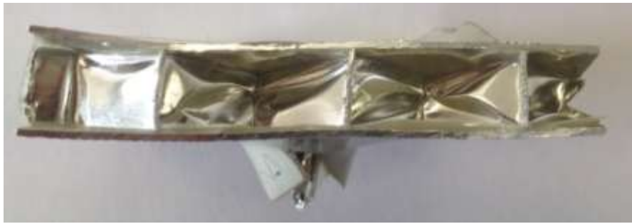
Figure 4.5: Deformed honeycomb due to out-of-plane compression loading.
