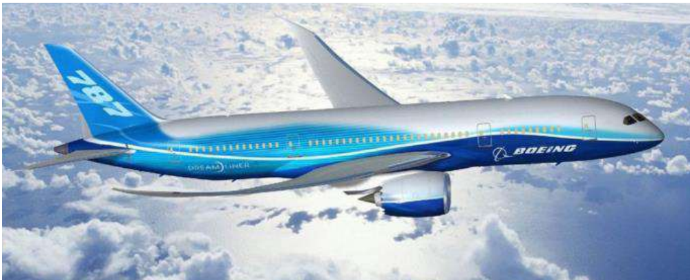
Figure 2.6: Over 50% composite commercial plane - Boeing's 787 Dreamliner.
