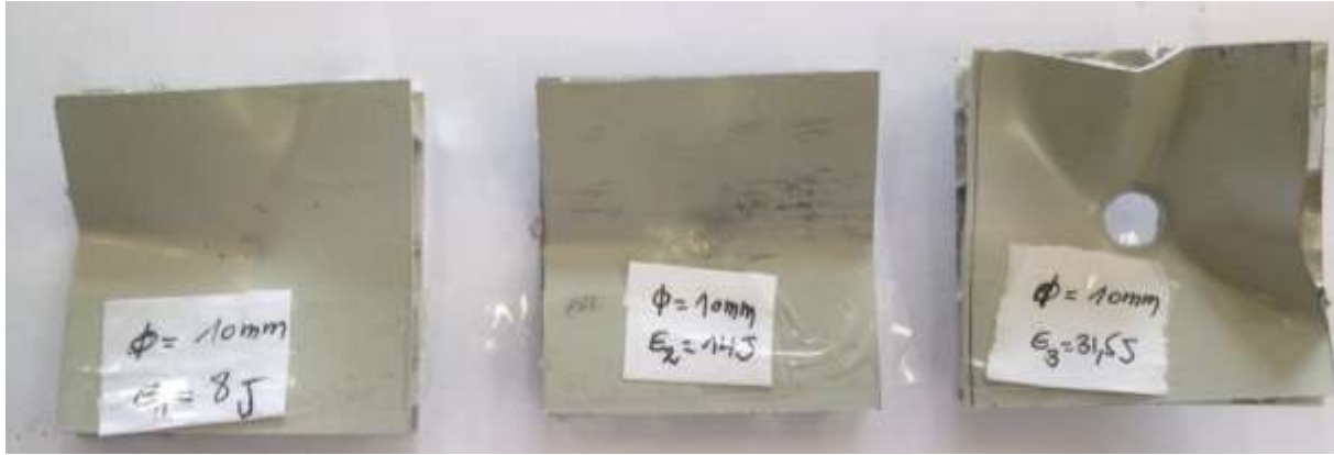
Figure 3.35: Photographs of deformed specimens at different impact energies (AHS d = 19.2 mm).
