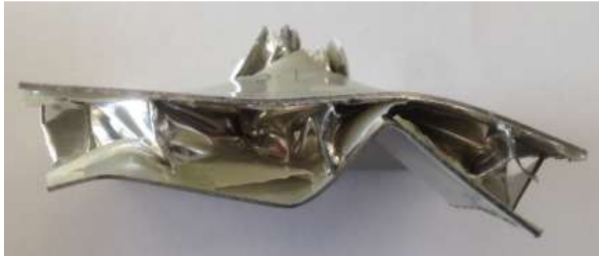
Figure 3.36: Total failure of AHS d = 19.2 mm
