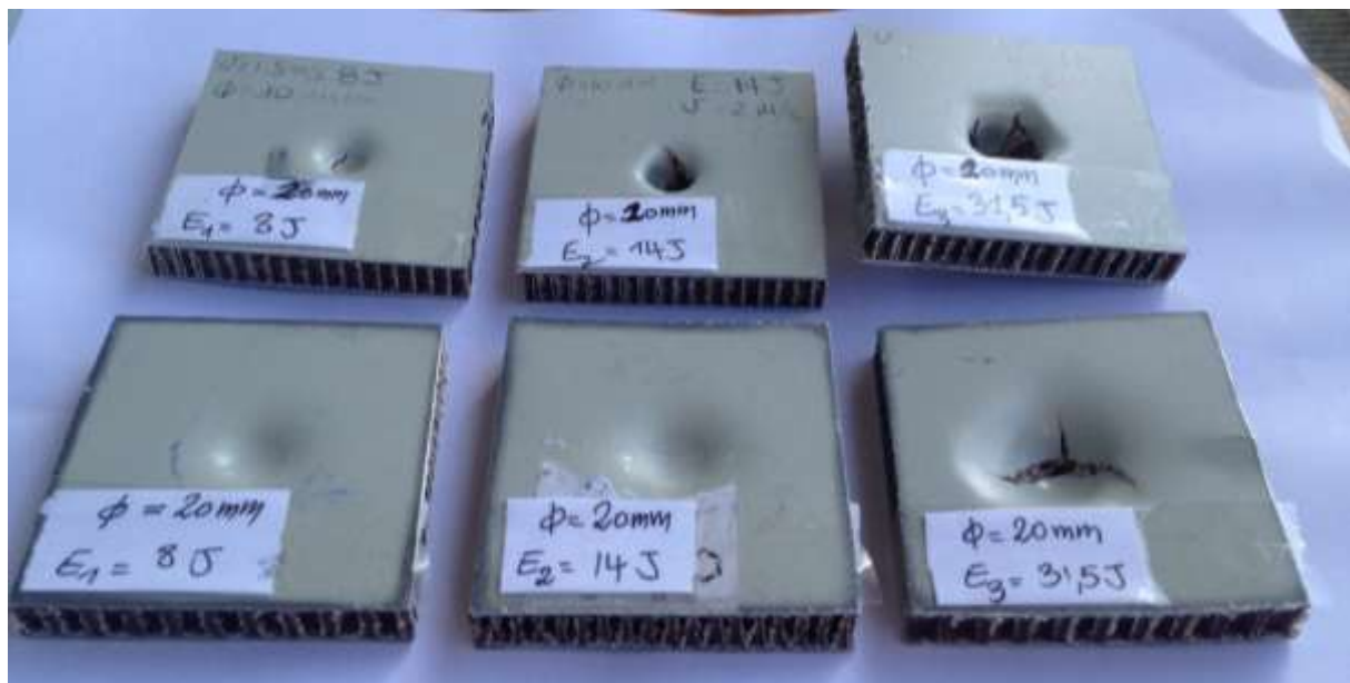
Figure 3.37: Photographs of deformed specimens at different impact energies (NHS d = 3.2 mm) for both impact (HS 20 et HS 10).
