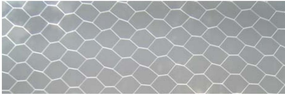
(a) Densité 55 kg/m<sup>3</sup>
