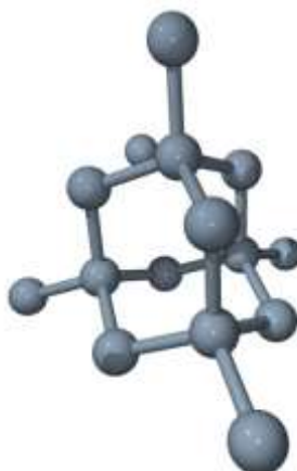
Figure 4 : Structure du diamant cubique [43] .
