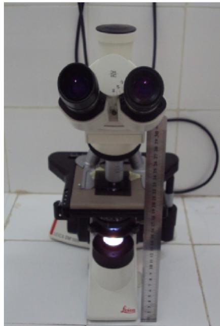
**Figure 3.8:** Microscope Leica DM1000.
