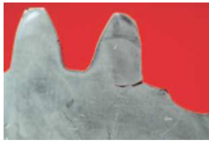
Figure I.2 : La rupture des dents [2]
